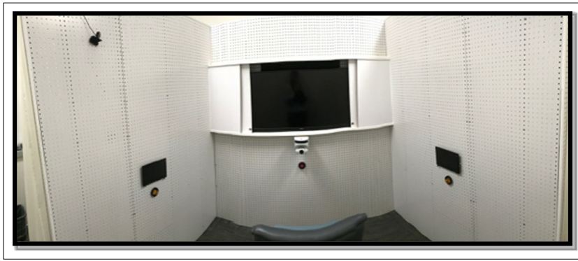
Fig. 2 A typical BITTSy setup. (The wide-angle camera lens makes the booth look curved, but it is actually a square with three walls and an open back.) The front panel has a large screen that can be used for central fixation or preferential looking studies; there are doors to the side that can close and cover the central monitor when not in use. Just under the monitor is a camera, and below that a central light, used for HPP studies. The two side panels (slightly distorted because of the use of a fisheye camera) each have a small monitor (for conducting HPP studies with video images) and a light (for standard HPP) mounted at the height of
